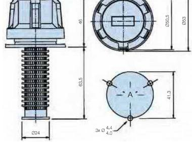
Note: Form 3 off tank mounting holes between Ø4.0 and Ø4.4mm (dependent on the material and thickness – see chart for guide) equispaced on 41.3 P.C.D. to suit No. 10 thread forming screws supplied.
