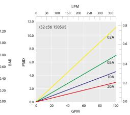
Correct for other fluids by multiplying new viscosity in cSt/32 (SUS/150) x new S.g./0.9
