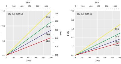
Correct for other fluids by multiplying new viscosity in cSt/32 (SUS/150) x new S.g./0.9
