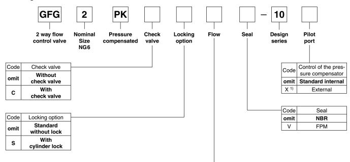
Code Flow [l/min] 0.6 0.015 to 0.6 1.0 0.015 to 1.0 1.6 0.015 to 1.6 3.2 0.025 to 3.2 6.3 0.025 to 6.3 12.0 0.080 to 12.0 18.0 0.080 to 18.0
